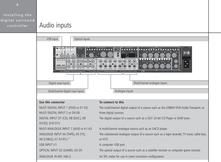
\* A4-A6 can be used as MULTI ANALOGUE INPUT 2 to connect to a second multichannel analogue source such as an SACD player.
