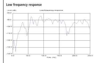
Shows the loudspeaker-room response to a low frequency sine wave, swept between 0 and 250Hz. The ideal low frequency response would be smooth. A peak in the response indicates a resonance at the corresponding frequency. A dip in the response indicates absorption or cancellation at the corresponding frequency.
