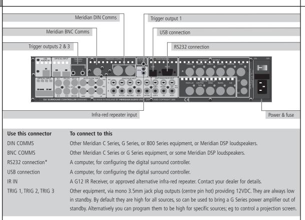
\*A second RS232 socket is provided on the front panel, and a switch allows you to select the active connector.
